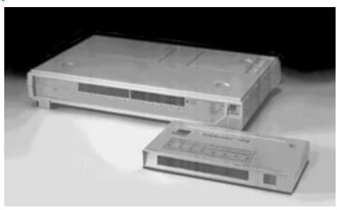
LinkBuilder TP/8 and LinkBuilder TP/12 Ethernet hubs put flexibility and quality design comfortably within the budget of a standalone, small office network. Simple to install and use, they are ideal for LANs with no on-site network support.
